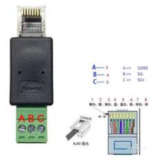
It is a simple conversion from RJ45 connector to a 3-screw terminal connector. The text: "SGND", "SG+" and "SG-" is placed on the removable connector.
